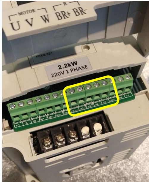
Fig.1 Find control input terminal X1,X2...X5 & COM under the bottom cover
