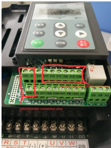
Fig.1 Open the lid, find the digital input terminals (DI1, DI2... DI5).
